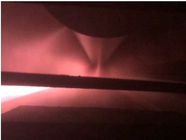
Figure 3. Unpowered magnetron affecting current flow.
