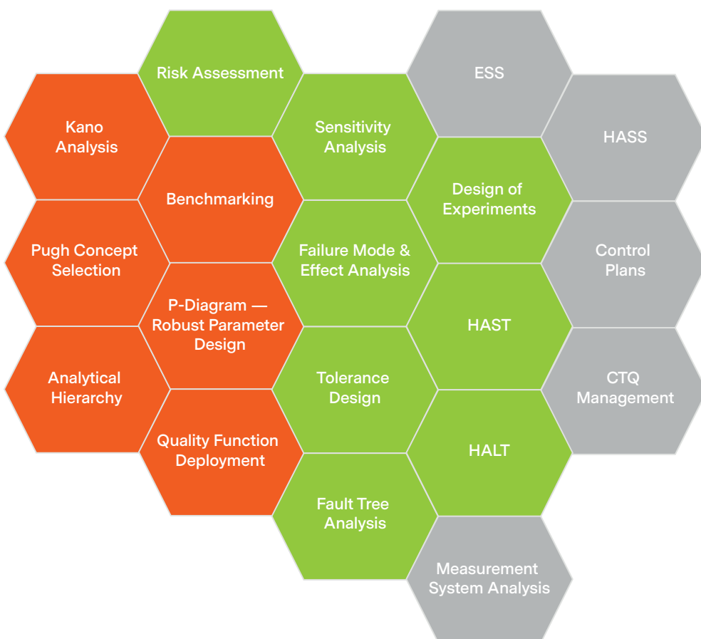
Figure 4. DfR tools; tools in different colors signify their typical use at various phases of product development
