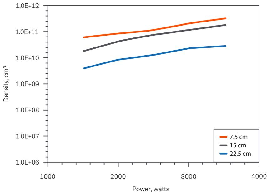
Figure 4. Nitrogen density versus power at various positions downstream.
