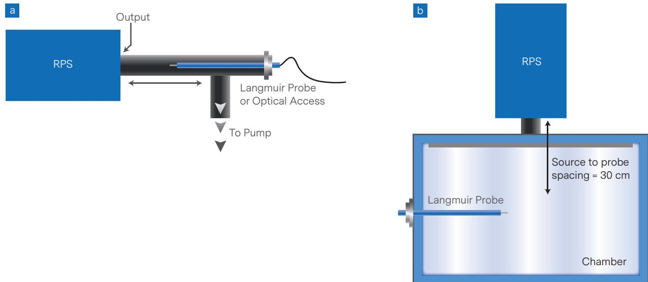
Figure 1. Configurations used for testing a) downstream projection into a confined space and b) projection into open-volume downstream chamber.
