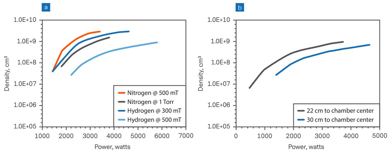
Figure 5. a) Projected density to the center of an open-volume chamber for nitrogen and hydrogen for source to probe spacing of 30 cm; b) projected density for hydrogen at 0.5 Torr showing the impact of reduced source to chamber/probe spacing.
