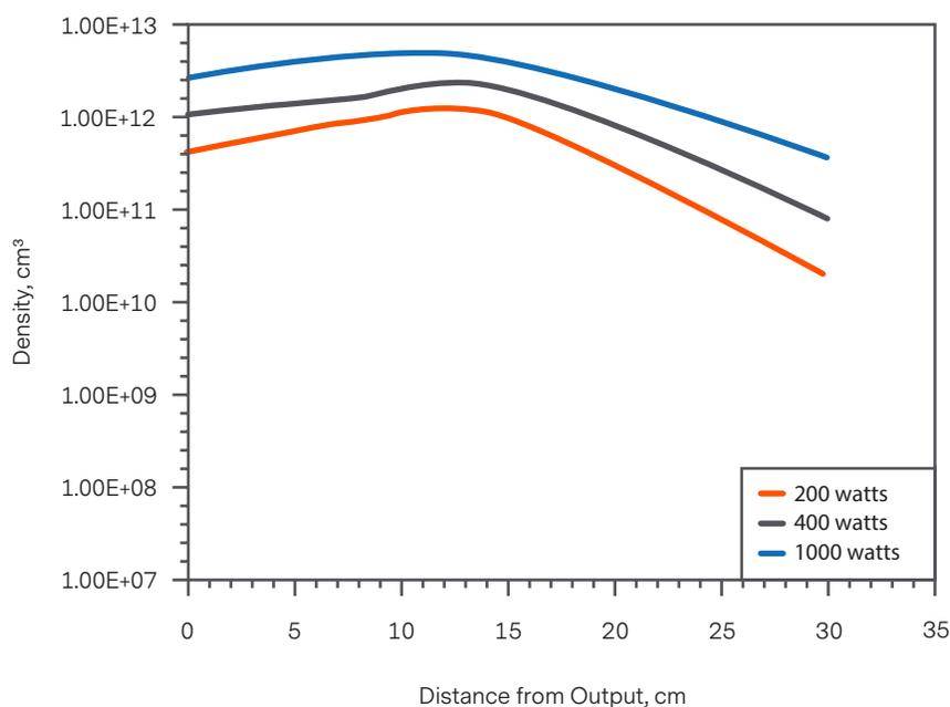
Figure 2. Plasma density for argon measured in the confined space downstream from the VFH RPS source.
