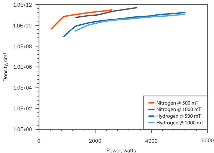
Figure 3. Nitrogen and hydrogen density at 15 cm downstream within confined volume.
