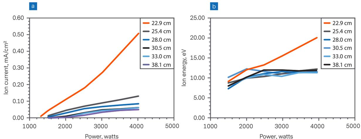
Figure 8. a) Ion current and b) energy projected to the downstream chamber as a function of VHF RPS power.
