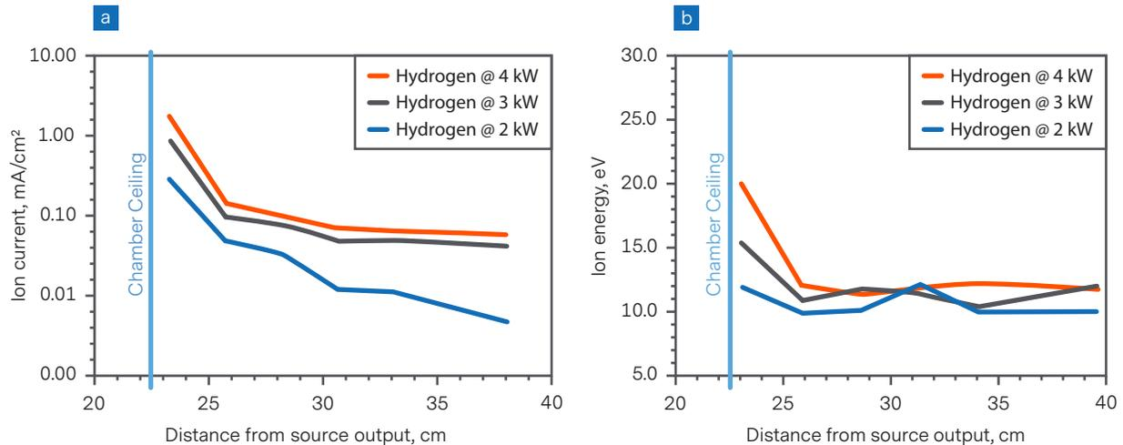
Figure 7. a) Ion current and b) ion energy projected from remote plasma source into large volume downstream chamber.
