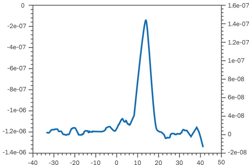
Figure 6. IEDF for hydrogen plasma projected to downstream chamber operated at 500 sccm, 300 mT and 3000 watts.
