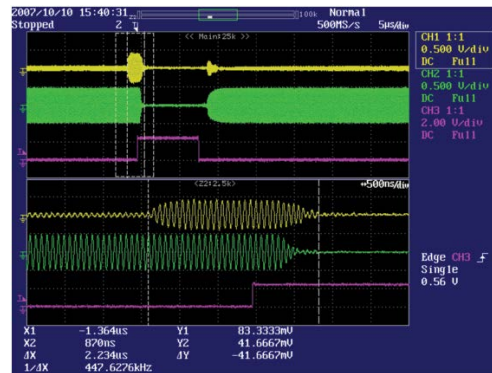
Sudden change in reflected power indicating an arc; Rapid output power shutdown. All arc management parameters are user-selectable.
