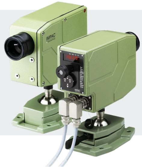
The Impac® IS 12-AI is a version of the pyrometer IS 12, specially designed for the measurement of aluminum. The robust die-cast housing with protection class IP 65 is designed for the use in industrial environments. The parameters of this digital instrument can be set directly via push buttons on the rear side of the instrument. The built-in digital display indicates the corresponding parameters or the actual temperature reading in measuring mode.
