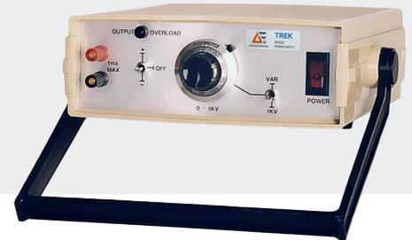
The Trek® 605A is a high voltage reference supply designed to provide precise control of output voltages in the range of 0 to +1 kVDC or 0 to -1 kVDC with an output current range of 0 to  $\pm 1$  mADC. The Trek 605A provides two modes of operation: a fixed mode providing a constant +1 kV or -1 kV output, and a variable mode providing variable control of the output voltage with a one (1) volt resolution over a range of 0 to  $\pm 1$  kV.
