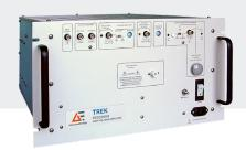
The Trek® PZD2000A is a wide bandwidth, high voltage power amplifier used for precision high power applications. The amplifier incorporates an all-solid-state design for high reliability and low-noise operation. Its four quadrant output stage sinks as well as sources load current throughout the output voltage range, thus achieving accurate output response and high slew rates, even into highly capacitive loads.
