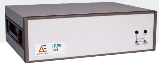
The Trek® 609B-3 is a DC-stable high voltage power amplifier. The four-quadrant, active output stage sinks or sources current into reactive or resistive loads throughout the output voltage range. This output is essential to achieve an accurate output response and high slew rate demanded by a highly capacitive or reactive loads. It is configured as a non-inverting amplifier, an inverting amplifier, or as a differential amplifier. Different input configurations can be wired into the unit.
