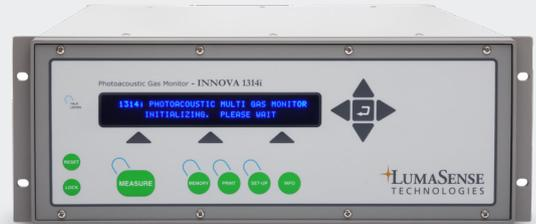
The Innova® 1314i Photoacoustic Gas Monitor is a highly accurate, reliable, and stable quantitative gas monitoring system. Its measurement system, based on the photoacoustic infrared detection method, is capable of measuring almost any gas that absorbs infrared light.
