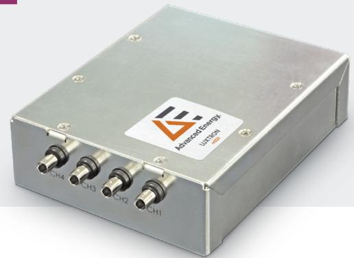
The Luxtron® m924 module uses Fluoroptic® technology, based on a temperature sensitive phosphorescent sensor attached to the end of an optical fiber. The complete m924 OEM solution consists of the electronics module assembly plus Luxtron probes and accessories. The system provides precise and repeatable in-situ temperature measurements for control of processes involving RF, EMI, magnetic fields and high voltages.
