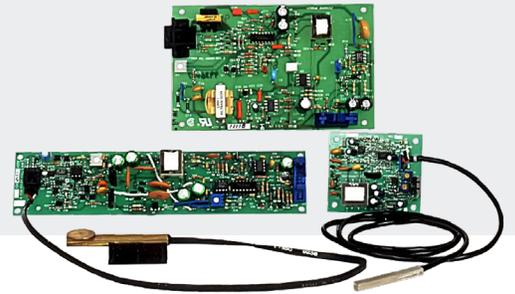
Trek® non-contacting on-board electrometers, commonly referred to as on-board controllers provide accurate, drift-free, highspeed, low-noise measurements of electrostatic potentials in a low cost unit for OEM electrophotography applications. These OBCs have an operating mean time until failure rating of greater than 16,000 hours and been installed in the products of leading electrophotographic copier and printer manufacturers around the world.
