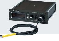
The Trek® 344 employs a field-nulling technique for non-contacting voltage measurement that achieves DC stability and high accuracy even if the probe-to-surface spacing changes. This permits measurements of either stationary or moving surfaces without the need to establish fixed spacing to maintain accuracy.
