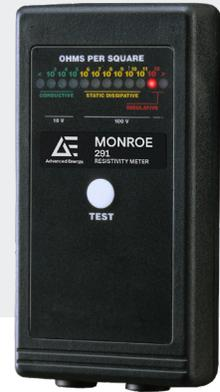
The Monroe 291 is a portable, battery-operated survey instrument for evaluating the resistive properties of static control products such as static dissipative packaging, flooring, or work surfaces over the range of  $10^3$  to  $10^{12}$  ohms or ohms per square
