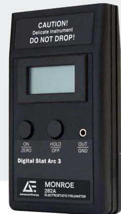
The Monroe 282-IS Digital Stat-Arc™ 2 and Monroe 282A-1 Digital Stat-Arc™ 3 are pocket-sized, non-contacting static meters for consistently accurate readings. Simply hold the instrument so the range finder LED beams from a non-pulsing circle indicating you're at exactly the right distance from the target for readings up to 20 kV.
