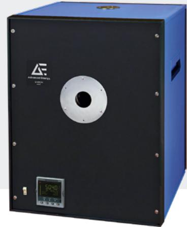
The Mikron® M300 is a high standard, precision blackbody calibration source designed with a unique uniformly heated spherical cavity that achieves a near ideal emissivity of 0.998 or better. The M300 will accurately deliver any temperature between 200 to 1150°C (392 to 2102°F). A convenient microprocessor-based, digital PID controller holds the selected temperature to within 1°C, ensuring high accuracy calibration.
