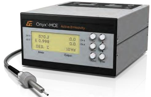
The **Onyx-MCE** is a multi-channel, non-contact optical fiber temperature pyrometer and incorporates a separate input for real-time reflectance measurement and active emissivity compensation. The system makes use of real-time emissivity measurement to precisely compensate for a material's change in emissivity during processing. The Onyx-MCE can be configured in a variety of measurement wavelengths and from single to dual measurement channels using separate optical sensors.
