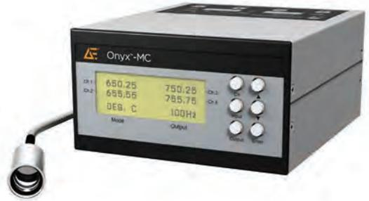
The **Onyx-MC** is a multi-channel, non-contact optical fiber temperature pyrometer that can be configured in a variety of measurement wavelengths based on a target material, required process temperature range, and working distances. Proprietary ambient temperature calibration technology ensures ongoing temperature measurement accuracy across a wide range of conditions by continuously monitoring each unit's internal temperature and automatically compensating for variations.
