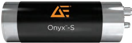
The **Onyx-S** is a single-channel, single-wavelength, non-contact infrared optical fiber pyrometer which can be configured to one of a number of measurement wavelengths based on target material, required process temperature, and working distances. Optional accessories include a water-cooling jacket, air-purge shower to protect against lens contamination, and specialized mounting accessories.
