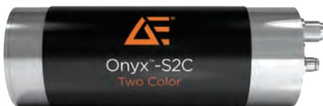
The **Onyx-S2C** is a two-color ratio, non-contact infrared optical fiber pyrometer which can be configured to one of a number of measurement wavelengths based on target material, required process temperature, and working distances. Optional accessories include a water-cooling jacket, air-purge shower to protect against lens contamination, and specialized mounting accessories.
