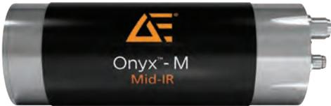
The Onyx™-M is a single-channel, single-wavelength, non-contact infrared optical temperature pyrometer which measures infrared energy being emitted from an object and converts this into temperature. The Onyx-M can be configured in a variety of measurement wavelengths based on target material, required process temperature range, and working distances. Optional accessories include a water-cooling jacket, air-purge shower to protect against lens contamination, and specialized mounting accessories.
