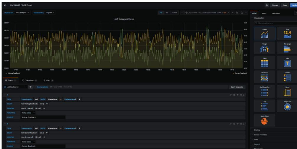
Construct a custom panel via a query builder: Choose which parameters to analyze; Apply mathematical methods, such as max, min, average, total, etc. to parameters; Choose visualization, such as Smith Chart, Bar gauge, Table, Graph, Stat, etc; Overlay data from different target units, and more.
