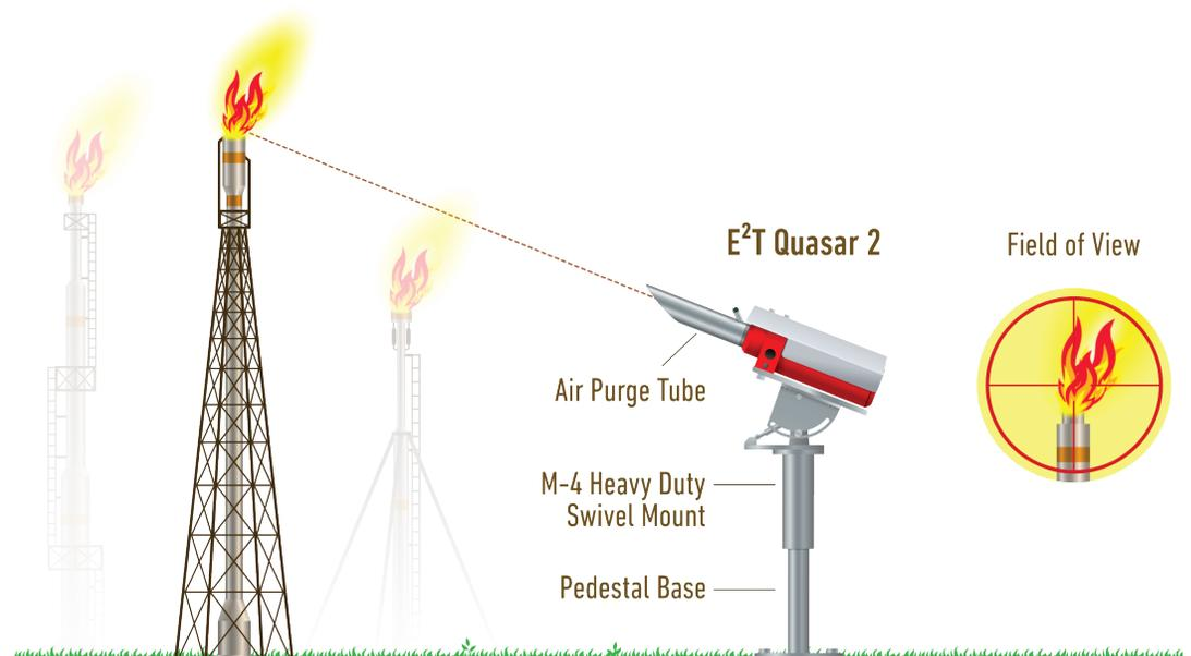
The E<sup>2</sup>T Quasar 2 M8100-EXP Flare Stack Flare Monitors provide continuous monitoring of flared gases from remote locations up to ¼ mile (400 m) away in nearly any climate condition. This solution is ideal for confirming compliance with government-set pilot monitoring requirements.
