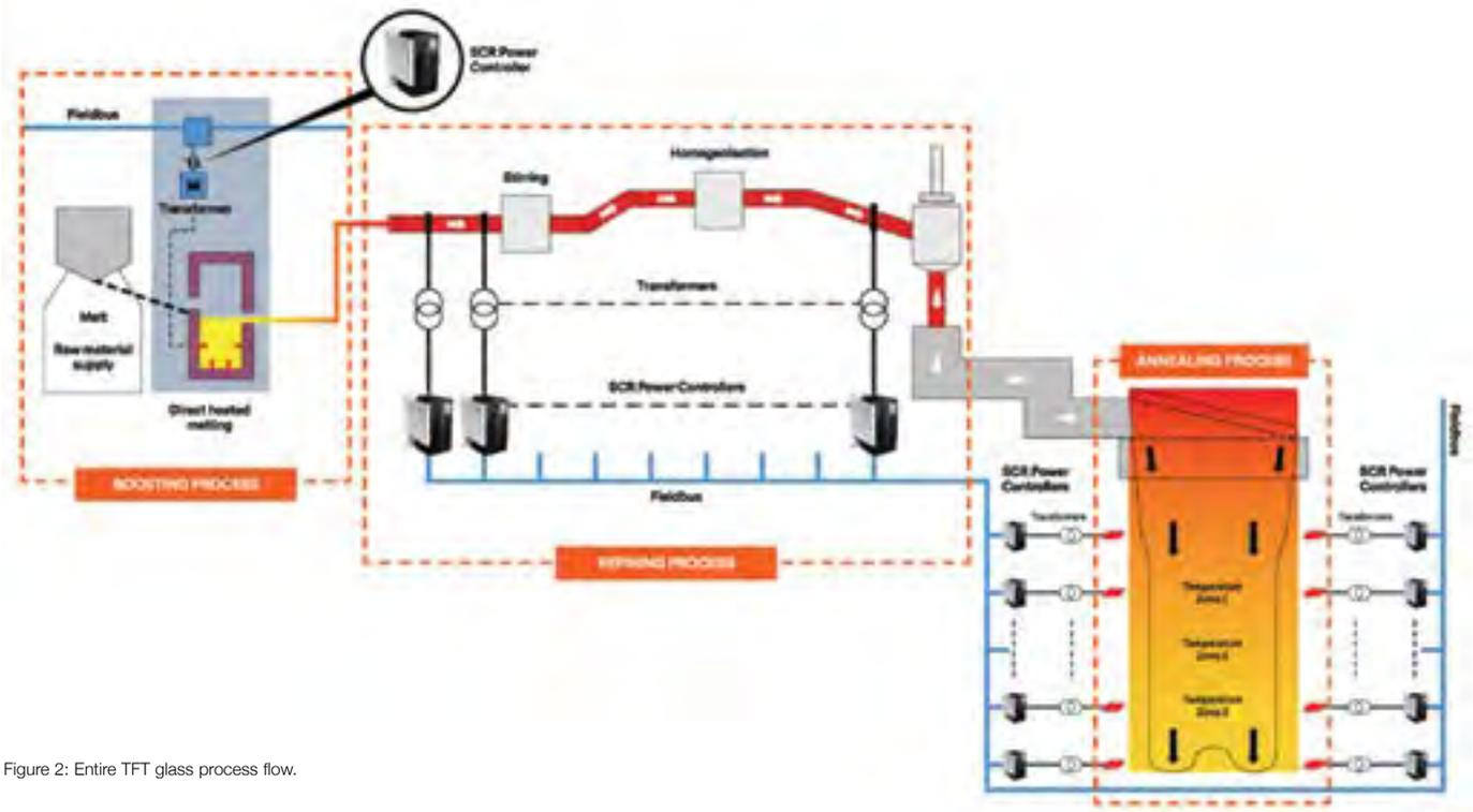
Figure 2: Entire TFT glass process flow.
