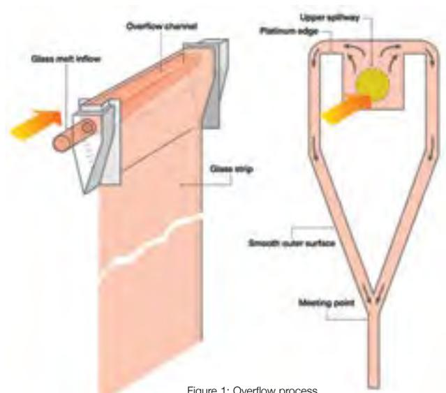
Figure 1: Overflow process.
