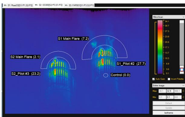
**Figure 1.** Software automates the monitoring of pilots and flares using thermal imaging camera streaming data, and continuously reports the status to a plant's distributed control system (DCS).
