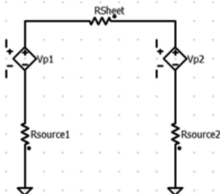
**Fig. 10** – Two-zone electrical model.
