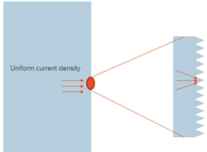
**Fig. 11** – Effect of edge on current density.
