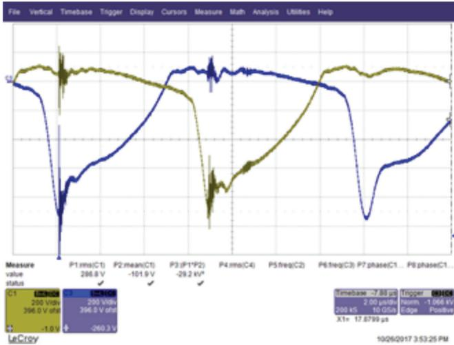
**Fig. 4** – Crystal output magnetron to ground.
