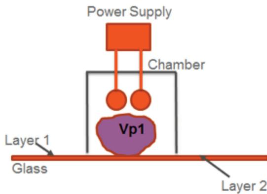
**Fig. 5** – Model of a single sputtering zone.
