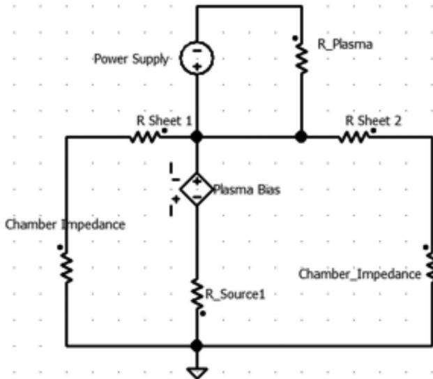
**Fig. 8** – Single zone electrical model
