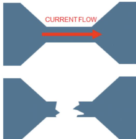
**Fig. 12** – Diagram of fuse element.
