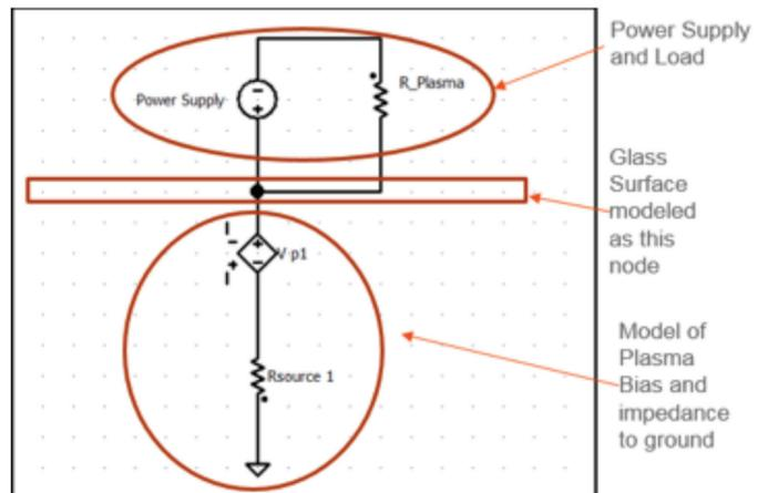
**Fig. 7** – Coating zone electrical model.
