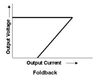
Foldback is a variation of the continuous approach. Once current limit is reached the convertor becomes a constant current supply. The value of current is a function of the degree of overload.
