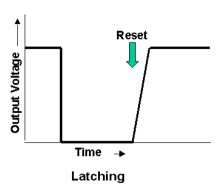
Latching overcurrent protection is by where the output voltage is pulled to zero but will not automatically recover until the system has been reset. This approach will not automatically recover but will wait for a system intervention.
