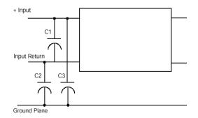
Convertor Z, needs three external components and a ground plane to meet Class B.
