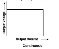
Continuous (also known as Brickwall) is where the output voltage goes to zero when the current trip point is reached. When the output overload is reached the unit will automatically recover.
