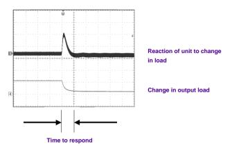
Transient response can be used to determine product stability from the transient response (to a good approximation).
