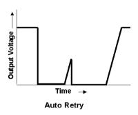
Auto retry is by where the unit will enter a hiccup-up mode. This is by where the unit will turn itself off and enter a wait mode. After a certain time, the unit will attempt to start itself up again, but will be unable to do so until the fault condition has been removed.
