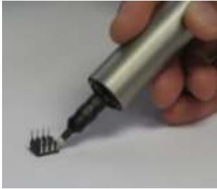
Figure 3. The probe contains the front end buffer amplifier
