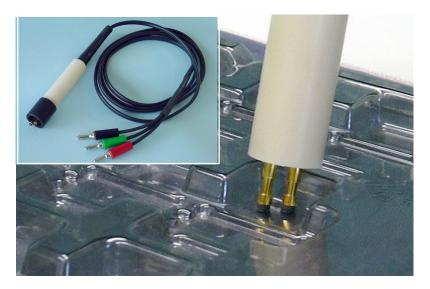
The Trek 152P-2P probe is used to perform accurate two point resistance measurements in the range of 10<sup>3</sup> to 10<sup>13</sup> ohms.
