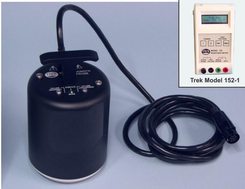
The Trek 152P-CR-1 Concentric Ring Probe is capable of measuring surface and volume resistance in materials as per IEC or ESDA standards. A three (3) position switch on the probe selects surface resistance or volume resistance measurements with either a guarded or unguarded outer electrode. (See page 2.)
