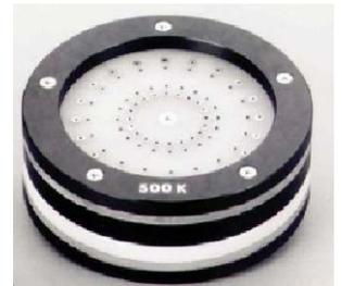
Surface Resistance Calibration Test Fixture
