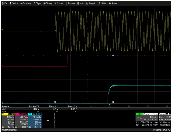
Figure 13: NGB150S15x Turn-On Delay via AC Mains V_{in} = 115\text{Vac} Load: I_O = 10\text{A} I_{SB} = 0.5\text{A} Ch 1: AC Mains Ch 2: V_{SB} Ch 3: V_O
