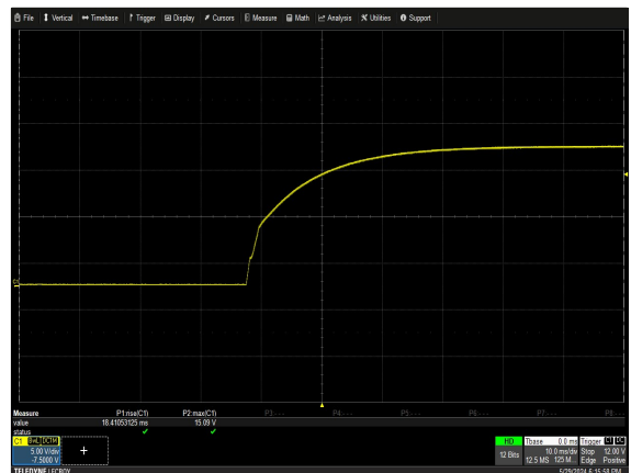
Figure 18: NGB150S15x Output Voltage Startup Characteristic V_{in} = 90\text{Vac} Load: I_O = 10\text{A} I_{SB} = 0.5\text{A} Ch 1: V_O
