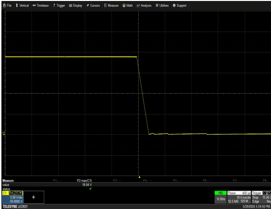
Figure 31: NGB150S19x Turn Off Characteristic Load: I_o = 7.9A I_{SB} = 0.5A Ch 1: V_O
