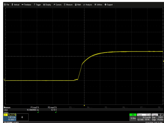
Figure 6: NGB150S12x Output Voltage Startup Characteristic V_{in} = 90\text{Vac} Load: I_o = 12.5\text{A} I_{SB} = 0.5\text{A} Ch 1: V_o
