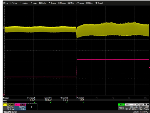
Figure 44: NGB150S24x Transient Response - V_o Deviation 50% to 100% load change 9.6mA/\mu s slew rate, V_{in} = 230Vac Ch 1: V_o Ch 2: I_o
