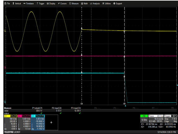
Figure 2: NGB150S12x Hold-Up Time V_{in} = 115\text{Vac} Load: I_o = 12.5\text{A} I_{SB} = 0.5\text{A} Ch 1: AC Mains Ch 2: V_{SB} Ch 3: V_o
