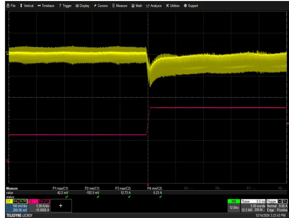
Figure 8: NGB150S12x Transient Response - V_o Deviation 50% to 100% load change 9.6mA/\mu S slew rate, V_{in} = 230Vac Ch 1: V_o Ch 2: I_o
