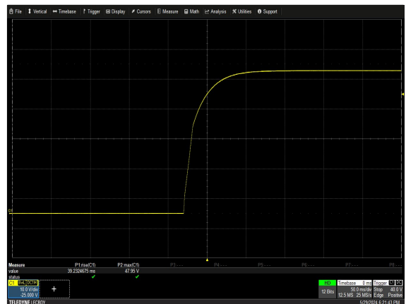
Figure 54: NGB150S48x Output Voltage Startup Characteristic V_{in} = 90\text{Vac} Load: I_o = 3.13\text{A} I_{SB} = 0.5\text{A} Ch 1: V_o
