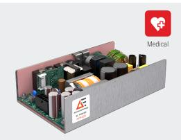
Advanced Energy's SL Power NCF425 CF rated\* medically approved AC-DC power supplies are available with a nominal main output of 12 V, 15 V, 24 V or 48 V. NCF425 series power supplies provide up to 425 W of output power with air flow. All models have output overvoltage, short circuit and overload protection and a 3.5 x 6 x 1.5 inch form factor.
