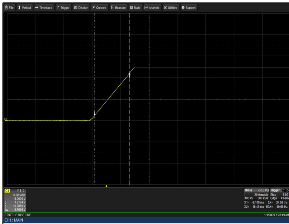
Figure 43: CSU2000AP-3-211 Output Voltage Startup Characteristic V_{in} = 180V_{ac} Load: I_o = 163.9A I_{SB} = 3.5A Ch 1: V_O
