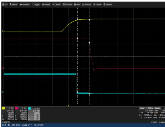
Figure 45: CSU2000AP-3-211 Turn Off Characteristic via PS ON Load: I_o = 163.9A I_{SB} = 3.5A Ch 1: PS ON Ch 2: V_O Ch 3: PWOK
