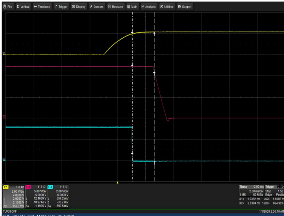
Figure 21: CSU2000AP-3-111 Turn Off Characteristic via PSOK Load: I_o = 163.9A f_{SB} = 3.5A Ch 1: PSOK Ch 2: V_O Ch 3: PWOK
