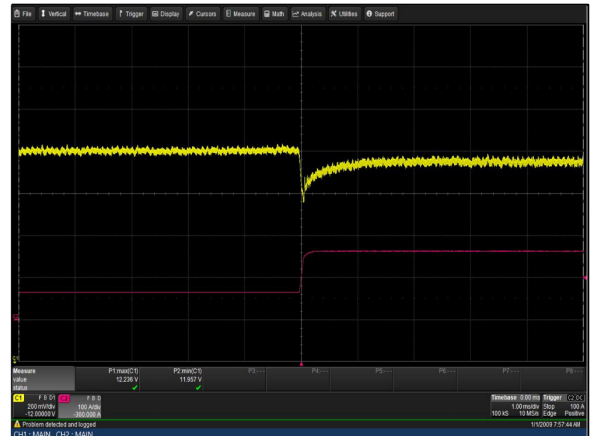
Figure 22: CSU2000AP-3-111 Transient Response - V_O Deviation 40% to 100% load change 0.5A/\mu s slew rate V_{in} = 230V_{ac} Ch 1: V_O Ch 2: I_o
