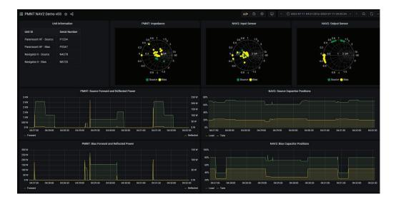
Example custom dashboard for monitoring match network and RF generator data with Smith chart:
