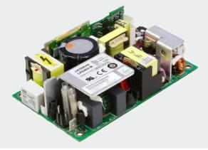
Advanced Energy's Artesyn LPS200-M series medicallyapproved AC-DC power supplies are available with a nominal main output of 5 V, 12 V, 15 V, 24 V or 48V. Auxiliary 12 V fan output is also provided. LPS200-M power supplies provide 125 Watts of output power with free air convection cooling or up to 250 Watts with 30 CFM of forced air. All models have a power factor of 0.99 typical and a 3 x 5 x 1.32 inch form factor.
