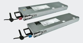
Advanced Energy's Artesyn CSZ3200FT-3 series is a closed frame, self-cooling power supply with regulated 55V PoE compliant main output and 3.3V standby output . Rated at 3200 W it is an 80 Plus Titanium supply with a high peak efficiency of 96%. Housed in an 1.58 x 3.95 x 14.55 inch rack-mounting package, the power supply is ideal for telecommunication environments. This series comes in two airflow versions – DC-connector to AC-connector and vice versa.
