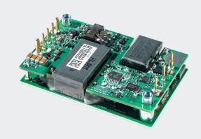
Advanced Energy's Artesyn AGQ500 series quarter-brick isolated DC-DC converters provides a single, regulated and low noise output. The AGQ500-48S50 has a 50V/10A output. It has a telecom input range of 36 to 75 VDC and is designed primarily for use with standard 48 V telecommunications equipment supplies. The converter's main application area is in low power and remote radio head (RRH) telecommunications applications.
