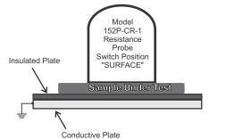
Resistivity - Resistance X Factor 10 = Resistivity
