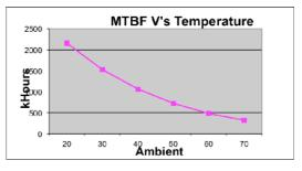
As you can see from Fig 1 above for every 10 degree rise in ambient temperature we see a 50% reduction in the calculated MTBF. This is clear if we work our way though the maths behind this.
