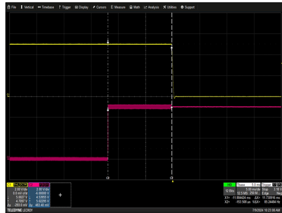
Figure 16: NP08W1-1ME0-00-A-0 Turn Off via Module Inhibit Load: I_o = 56A Ch 1: V_O Ch 2: Module Inhibit
