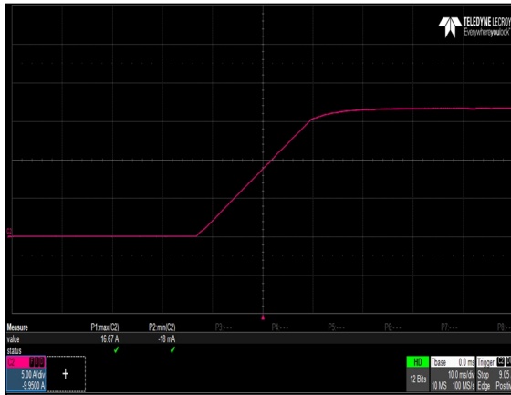
Figure 48: NP08W1-1MQ0-00-A-0 Output Current Startup Characteristic Load: R = 1.43 \text{ ohm} Ch 2: I_O
