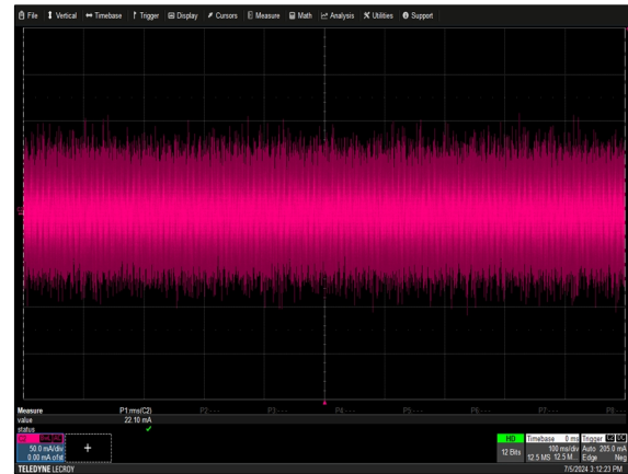
Figure 49: NP08W1-1MQ0-00-A-0 Ripple and Noise Measurement Load: R = 1.43 \text{ ohm} Ch 2: I_O
