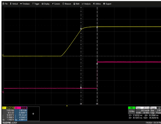
Figure 24: NP08W1-1ML0-00-A-0 Output Voltage Startup Characteristic Load: I_o = 33.3A Ch 1: V_O Ch 2: ISO_POWER_GOOD
