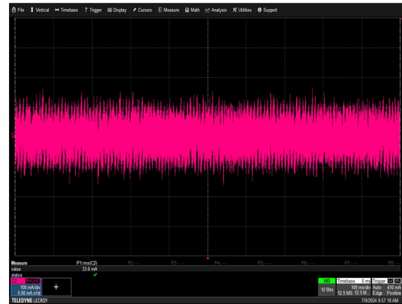
Figure 22: NP08W1-1ME0-00-A-0 Ripple and Noise Measurement Load: R = 0.08 ohm Ch 2: I_O
