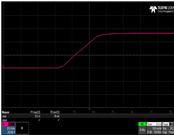
Figure 21: NP08W1-1ME0-00-A-0 Output Current Startup Characteristic Load: R = 0.08 ohm Ch 2: I_O
