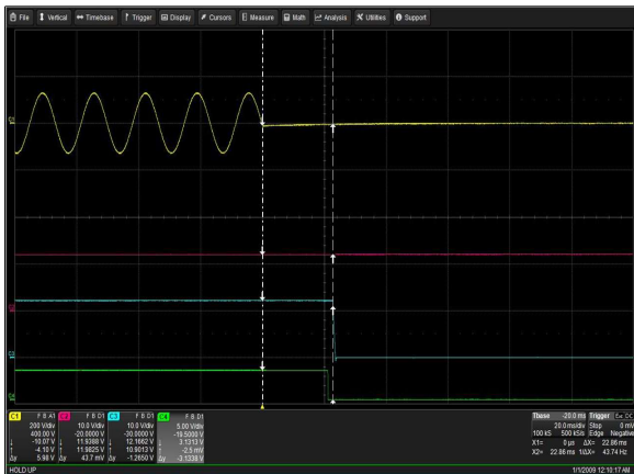
Figure 15: CSU2000AP-3-111 Hold-Up Time Vin = 90Vac Load: I O = 102.5A I SB = 3.5A Ch 1: AC Mains Ch 2: V SB Ch 3: V O Ch 4: PWOK
