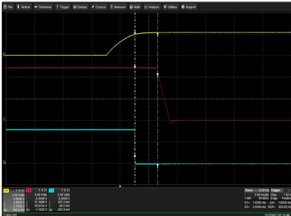
Figure 21: CSU2000AP-3-111 Turn Off Characteristic via PSON Load: I_o = 163.9A I_{SB} = 3.5A Ch 1: PSON Ch 2: V_o Ch 3: Pwok
