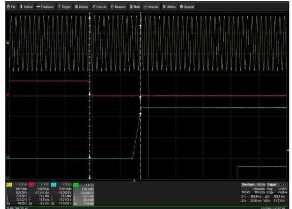
Figure 38: CSU2000AP-3-211 Turn-On Delay via PSON Vin = 180Vac Load: I O = 163.9A I SB = 3.5A Ch 1: AC Mains Ch 2: PSON Ch 3: V O Ch 4: PWOK
