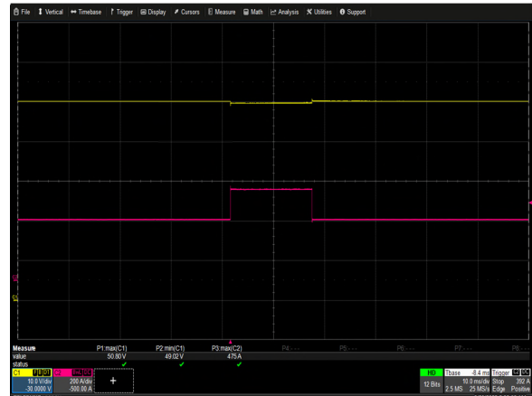
Figure 16: ORV3 Shelf Pulse Load (5 PSUs in the shelf) Vin = 400Vac(L-L) Io = 300A to 450A (16ms) single pulse Ch 1:Vo Ch 2: Io (slow rate: 5A/us)
