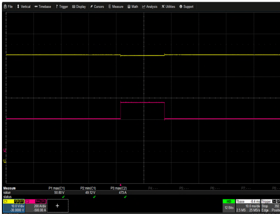
Figure 15: ORV3 Shelf Pulse Load (6 PSUs in the shelf) Vin = 400Vac(L-L) Io = 300A to 450A (16ms) single pulse Ch 1:Vo Ch 2: Io (slow rate: 5A/us)
