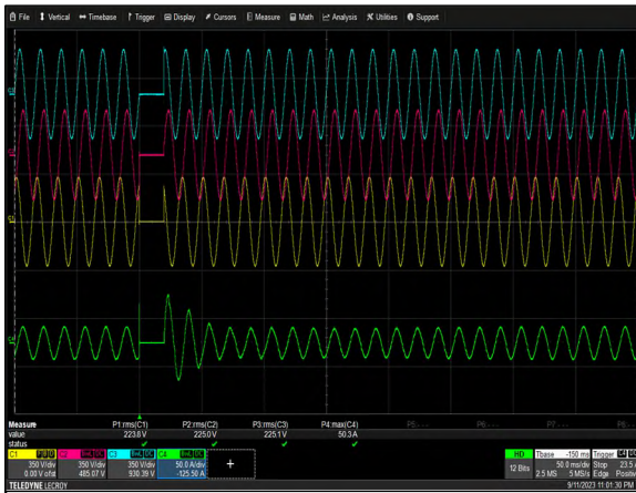
Figure 19: ORV3 Shelf Inrush Current Vin = 230Vac(L-N) (3 phases drop for 20ms) Io = 150A Ch 1: Vin (L1-N) Ch 2: Vin (L2-N) Ch3: Vin (L3-N) Ch4:lin
