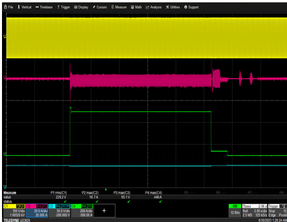
Figure 21: ORV3 Shelf Over Power/Current Protection Vin = 400Vac(L-L) Io = 432A(100ms) to 396A(9.9s) to 40A(1.14s) Ch 1:Vin Ch 2: lin Ch3:Vo Ch4:Io
