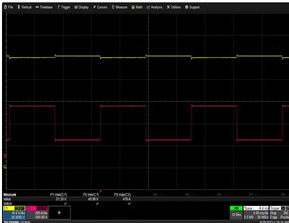
Figure 17: ORV3 Shelf Pulse Load (6 PSUs in the shelf) Vin = 400Vac(L-L) Io = 150A(8ms) to 450A (8ms) repetitive Ch 1:Vo Ch 2: Io (slow rate: 5A/us)
