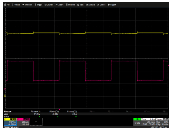
Figure 18: ORV3 Shelf Pulse Load (5 PSUs in the shelf) Vin = 400Vac(L-L) Io = 150A(8ms) to 450A (8ms) repetitive Ch 1:Vo Ch 2: Io (slow rate: 5A/us)
