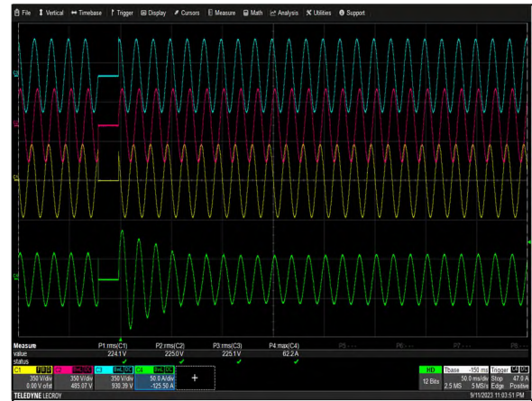
Figure 20: ORV3 Shelf Inrush Current Vin = 230Vac(L-N) (3 phases drop for 20ms) Io = 300A Ch 1: Vin (L1-N) Ch 2: Vin (L2-N) Ch3: Vin (L3-N) Ch4:lin
