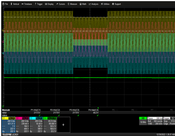
Figure 11: ORV3 Shelf Ride Through Test (6 PSUs in the shelf) Vin = 230Vac to 160V (1s) to 230Vac (L-N) Io = 300A Ch 1: Vin (L1-N) Ch 2: Vin (L2-N) Ch3: Vin (L3-N) Ch4:Vo
