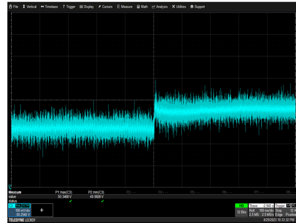
Figure 24: ORV3 Hot Swap Peak Deviation (Insert the 6th PSU) Vin = 400Vac (L-L) Io = 300A Ch 4: Vo (100mV/div, 100ms/div)
