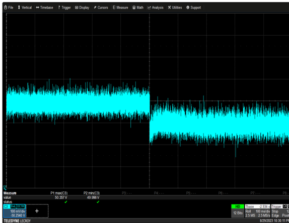
Figure 23: ORV3 Hot Swap Peak Deviation (Extract the 6th PSU) Vin = 400Vac (L-L) Io = 300A Ch 3: Vo (100mV/div, 100ms/div)
