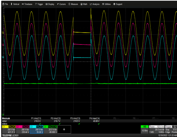
Figure 7: ORV3 Shelf Ride Through Test (6 PSUs in the shelf) Vin = 230Vac to 0V (20ms) to 230Vac (L-N) Io = 300A Ch 1: Vin (L1-N) Ch 2: Vin (L2-N) Ch3: Vin (L3-N) Ch4:Vo
