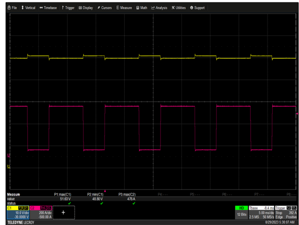
Figure 14: ORV3 Shelf Pulse Load (5 PSUs in the shelf) Vin = 400Vac(L-L) Io = 60A(3.75ms) to 450A (6ms) repetitive Ch 1:Vo Ch 2: Io (slow rate: 5A/us)
