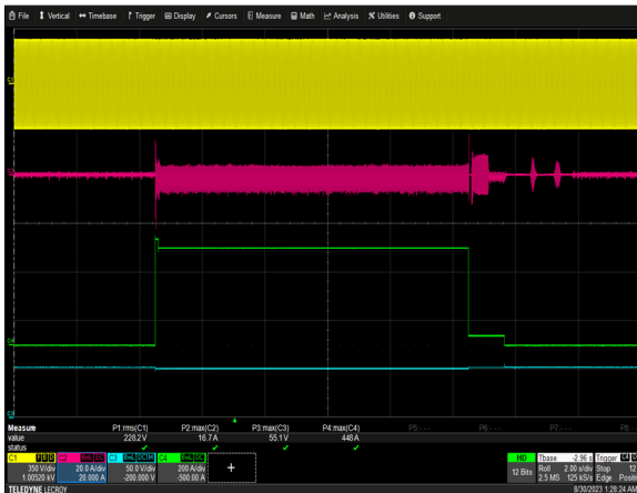
Figure 21: ORV3 Shelf Over Power/Current Protection Vin = 400Vac(L-L) Io = 432A(100ms) to 396A(9.9s) to 40A(1.14s) Ch 1: Vin Ch 2: Iin Ch 3: Vo Ch 4: Io
