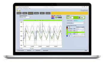
The TQCS software is used in combination with digital or analog pyrometers for recording and documentation of temperatures for every single processed piece on up to 30 machines simultaneously.
