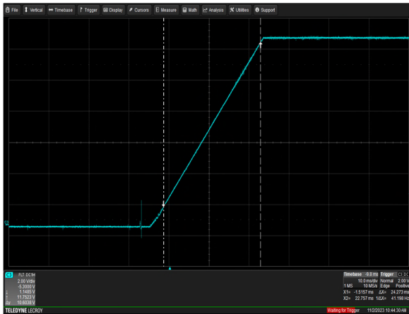
Figure 7: CSU1800AT-3-100 Output Voltage Startup Characteristic V_{in} = 90V_{ac} Load: I_o = 81.9A I_{SB} = 3.5A Ch 3: V_O
