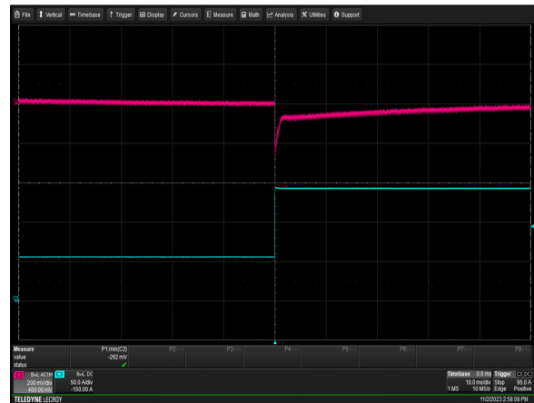
Figure 10: CSU1800AT-3-100 Transient Response - V_O Deviation 59A to 147.5A (40% to 100%) 1A/μs slew rate V_{in} = 230V_{ac} Ch 2: V_O Ch 3: I_o Output Cap: 2200μF
