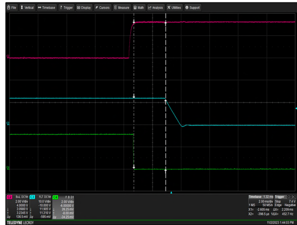
Figure 8: CSU1800AT-3-100 Turn Off Characteristic via PSON V_{in} = 90V_{ac} Load: I_o = 81.9A I_{SB} = 3.5A Ch 2: PSON Ch 3: V_O Ch 4: PWOK
