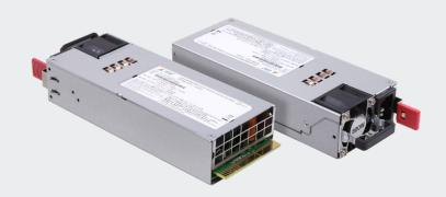
Advanced Energy's Artesyn CSU800AP power supply is housed in a 1U high rack-mount enclosure measuring just 2.89 x 7.28 inches (73.5 x 185.0 mm). This form factor is significantly narrower and shorter than that of similarly rated earlier generation power supplies - freeing up valuable system space - and is achieved by use of the latest power switching technology and high density component packaging techniques. This form factor conforms to the standard market's Common Redundant Power Supplies.
