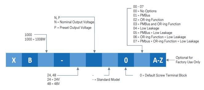
**Example 1:** XB1000-24N-000 = Suitable for BF-rated applications 1000 W, 24 V, output with no options
