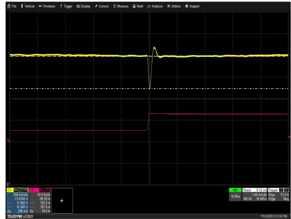
Figure 10: CSU800AP-3-600 Transient Response - V_O Deviation 40% to 100% load change 0.5 A/uS slew rate V_{in} = 230 \text{ Vac} Ch 1: V_O Ch 2: I_O
