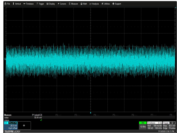
Figure 8: CSU800AP-3-600 Ripple and Noise Measurement Load: I_O = 66.7 \text{ A} I_{SB} = 3 \text{ A} Ch 3: V_O
