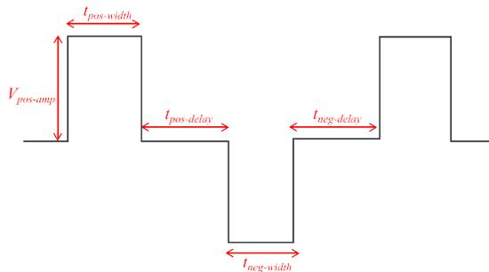
Fig. 7: An example of poorly-defined amplitude and timing definitions.
