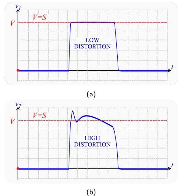
Fig. 11: A single rectangular pulse with perfect accuracy and (a) low distortion and (b) high distortion.
