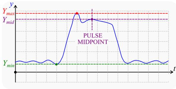
Fig. 8: The MAXIMUM  $Y_{max}$ , MINIMUM  $Y_{min}$  and MID-POINT MAGNITUDES  $Y_{mid}$  of a PULSE  $y(t)$ .
