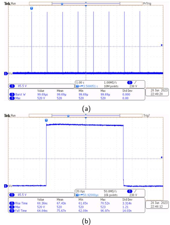
Fig. 13: Pulsed output for skin ECT using ESOP at  $f_p = 1$  Hz depicting an entire (a) BURST and (b) a single PULSE.
