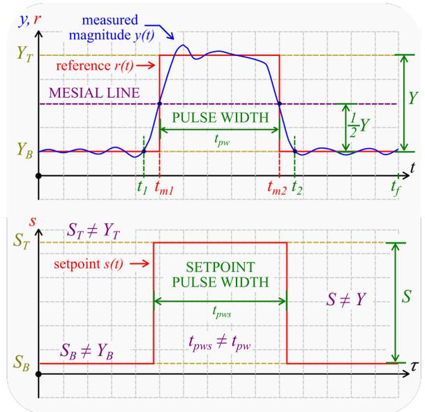
Fig. 9: The REFERENCE WAVEFORM  $r(t)$  and SETPOINT WAVEFORM  $s(\tau)$  of a RECTANGULAR PULSE with MAGNITUDE  $y(t)$ .
