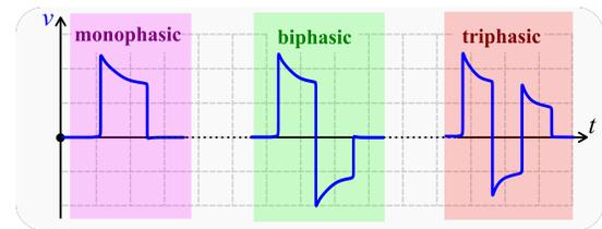
Fig. 5: The meaning of monophasic, biphasic and triphasic defibrillation waveshapes.
