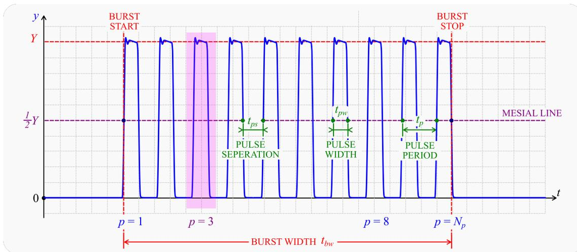
Fig. 10: A single UNIPOLAR BURST  $y(t)$ .
