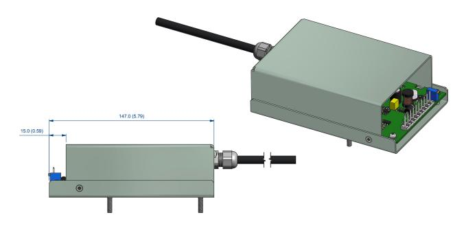
MOUNTING: 2 OFF M4 STUDS; LENGTH AND POSITION AS SHOWN DIMENSIONS mm (in)
