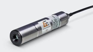
The Impac® IN 300 is a stationary pyrometer for non-contact temperature measurement of non-metallic surfaces or painted, coated, or anodized metals. The very small housing dimensions enable the integration of the pyrometer into compact production machines, the two-wire technique enables very easy electrical connection. The solid and robust design of the instrument guarantees high operational safety even in rough industrial environments.
