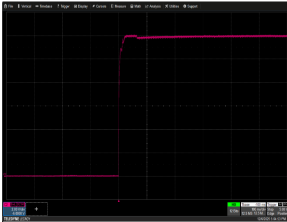
Figure 7: CSU3200AT-3-3M0 Output Voltage Startup Characteristic V_{in} = 240V_{ac} Load: I_o = 262.3A I_{SB} = 3A Ch 1: V_O
