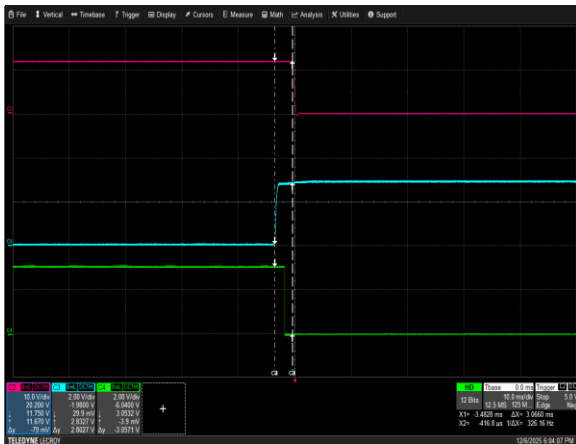
Figure 9: CSU3200AT-3-3M0 Turn Off Characteristic via PSOn Load: I_o = 262.3A I_{SB} = 3A Ch 2: V_O Ch 3: PSOn Ch 4: PWOK
