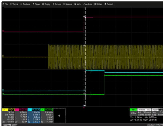
Figure 5: CSU3200AT-3-3M0 VIN_GOOD Assert Characteristic
