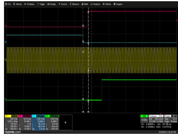
Figure 2: CSU3200AT-3-3M0 Turn-On Delay via PSON
