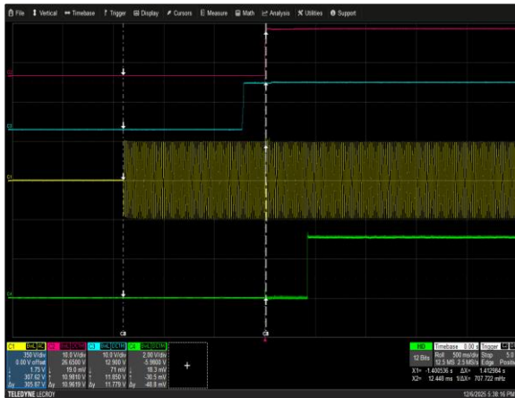
Figure 1: CSU3200AT-3-3M0 Turn-On Delay via AC Mains
