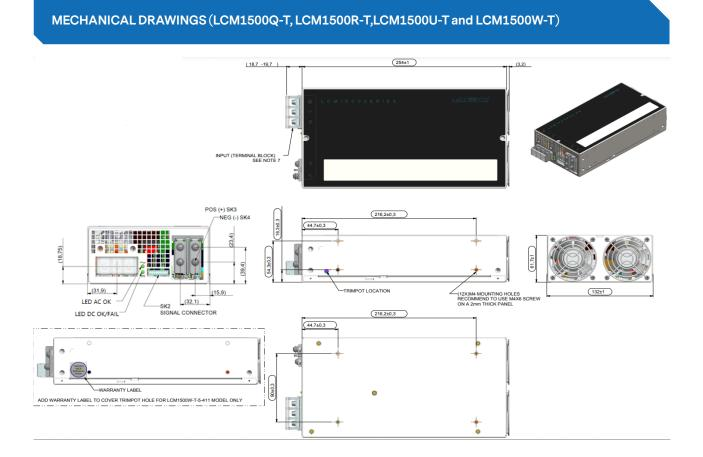
Notes: MOUNTING LOCATIONS SCREW PENETRATION DEPTH IS 4.6 mm MAX. RECOMMENDED SCREW TORQUE: M3.5 x 0.6P = 6 - 8kgf-cm M4.0 x 0.7P = 8 - 10kgf-cm
