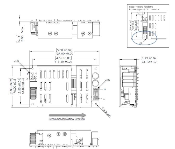
Note 1 - Dimensions: W: 3.0" x L: 5.0" x H: 1.37" (W: 76.2 mm x L:127 mm x H: 34.9 mm).
