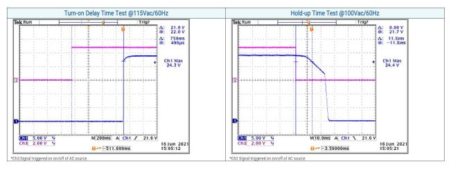
Performance data results for SLB300S24C, Class II with 24 V output at 25°C. Data for other voltages, Class II and other temperatures available upon request.
