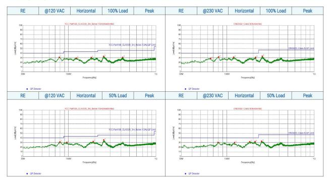
Note - Conducted and radiated emissions plots show measurements with resistive loads according to the IEC/EN/UL standard's requirements. EMC performance can be impacted by system level design, integration, or associated connections with additional wires and/or devices. Contact AE for support with system level EMC compliance needs.
