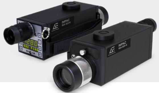
The Impac® IGA 315-K infrared thermometers are high-quality, battery driven portables for non-contact temperature measurement. The instruments feature a modified optical path for easily targeting the nozzle brick through a small space from the oven roof after opening the heating flue. With the high-quality focusable optics, accurate measurements can be made at distances between 1 and 12 m.
